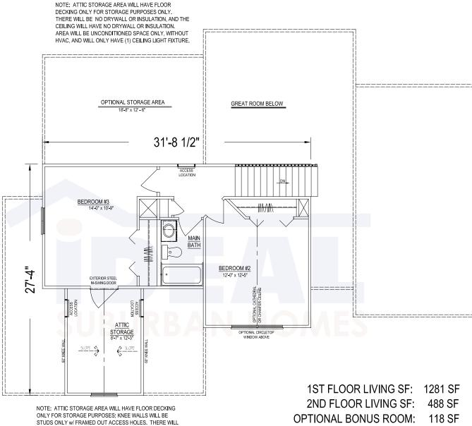
BE NO DRYWALL OR INSULATION, AND THE CEILING WILL HAVE NO DRYWALL OR INSULATION. AREA WILL BE UNCONDITIONED SPACE ONLY, WITHOUT HVAC, AND WILL ONLY HAVE (1) CEILING LIGHT FIXTURE. THIS AREA MAY BE UPGRADED TO A SEMI-FINISHED OR COMPLETELY FINISHED BONUS ROOM TO MEET CUSTOMERS NEEDS.
